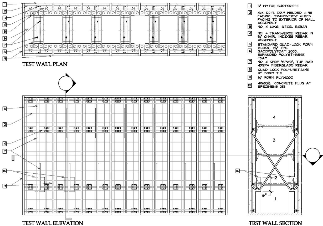
Figure 2 Test wall assembly
