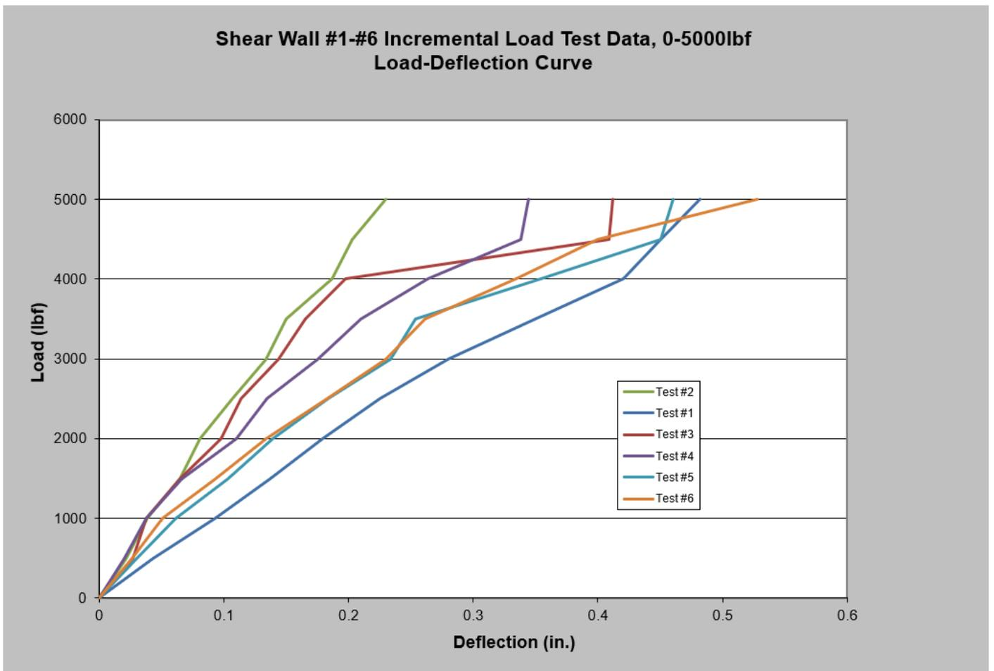
Lateral displacement of upper concrete panel relative to lower concrete panel when sample wall is loaded in shear.
