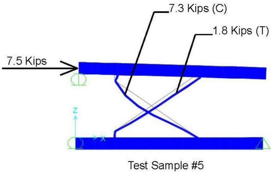
Figure 8b Load deflection curve and FEM sample 5
