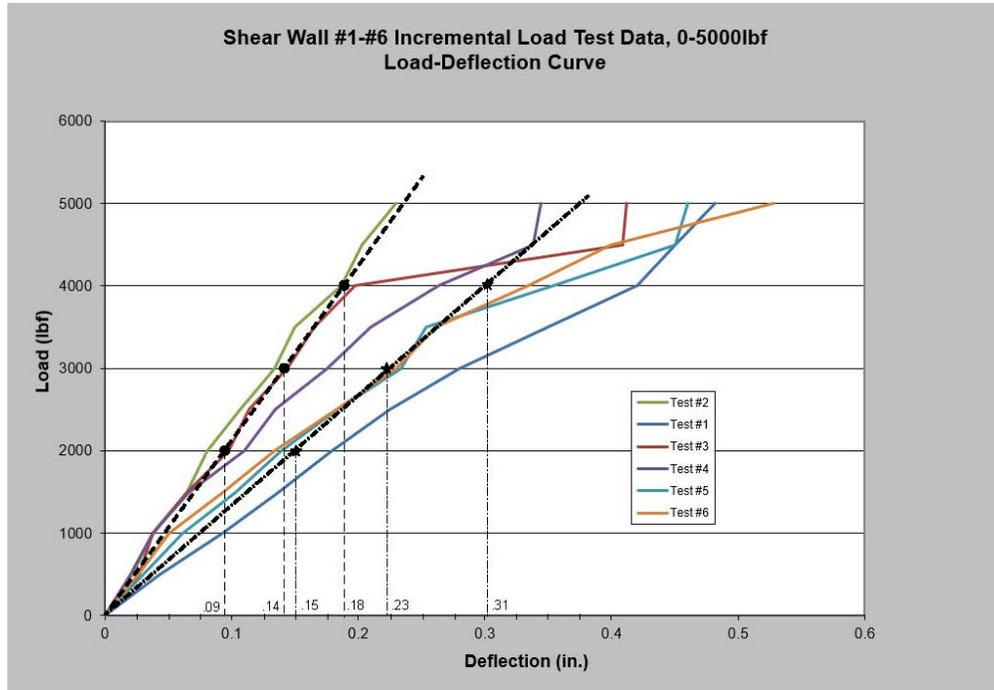
Figure 7a AME load deflection curves with FEM overlays
