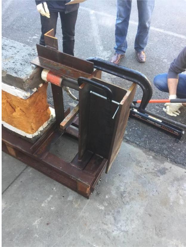
**Figure B1a.** Steel frame test apparatus with sample being loaded.
