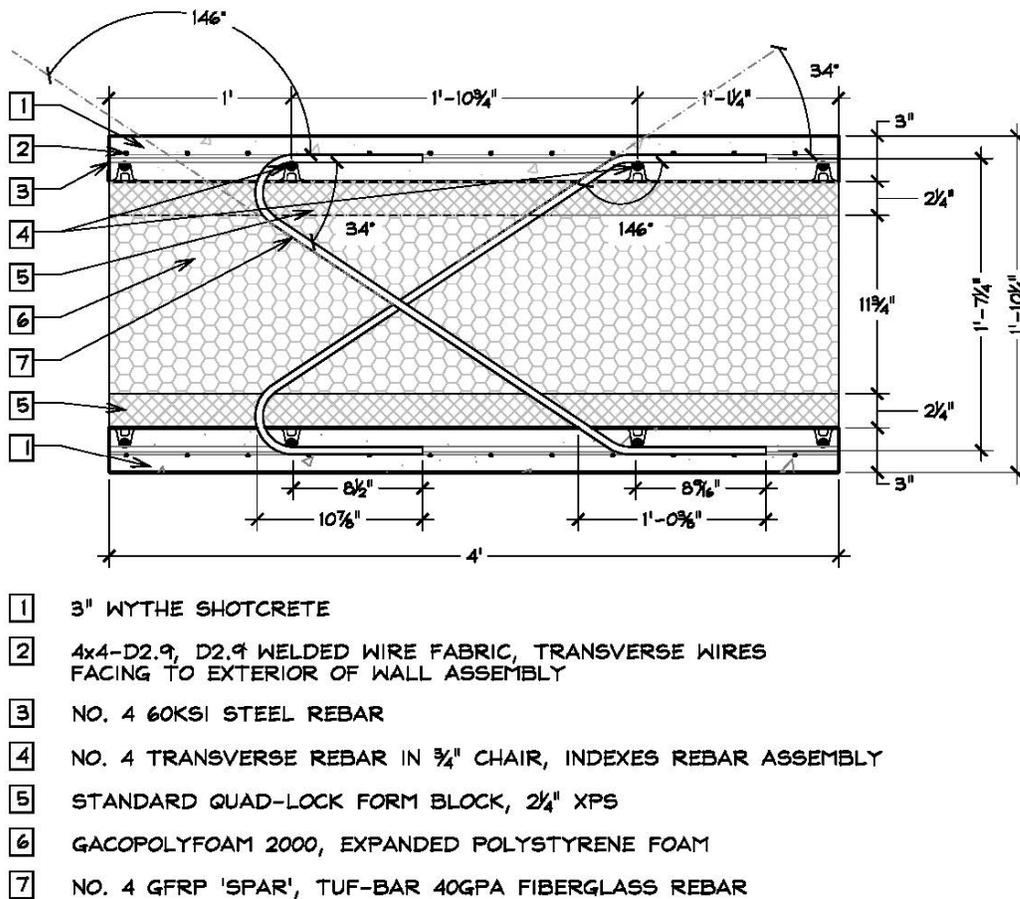
Figure 1 Cross section of test specimen
