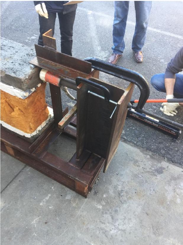
Figure 4b Steel frame testing apparatus with sample being loaded
