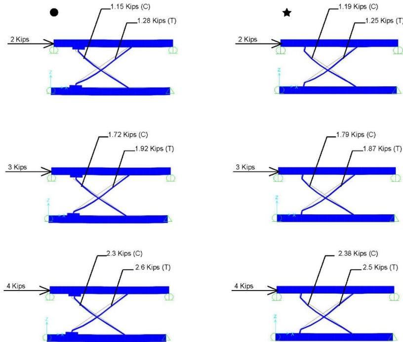
Figure 7b FEM models at different ram forces
