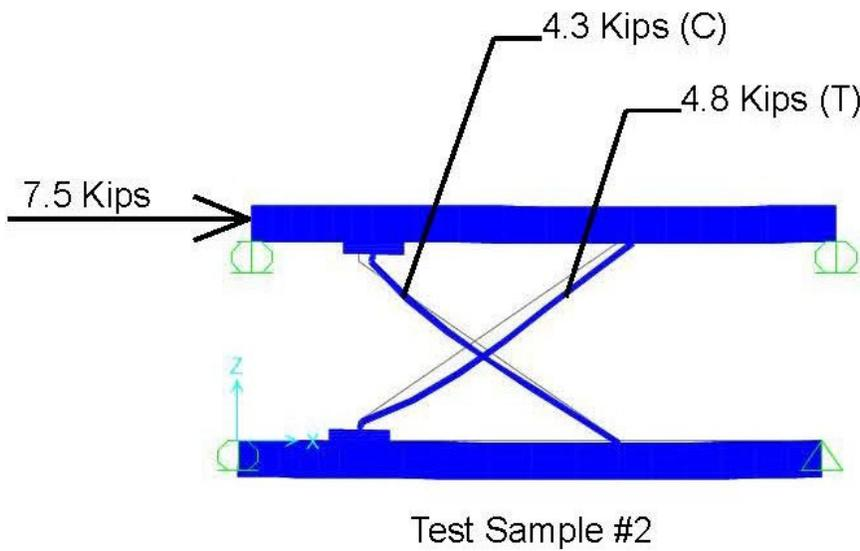
Figure 8a Load deflection curve and FEM sample 2
